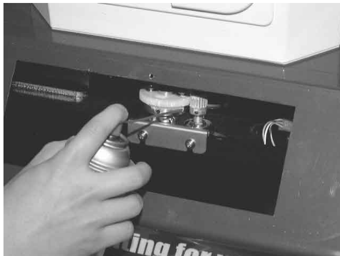
PHOTO 10. 4 a GEAR MESH PORTION, VR GUIDE SLIDING PORTION
