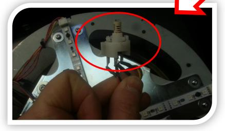
Remove the D-Pad molding
