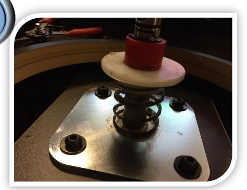
Push the plate up and down a few times to work in the grease.
