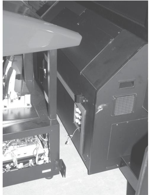
The connector panels are to the front left and right of the DLP projector. Besides the connector panel connectors, there is an earth wire inside the rectangular hole on the left side. Inside the rectangular hole on the right side, there is a wire for the yellow connector.
