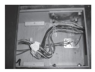
**7** Fasten the cable down with the 3 cord clamps.
