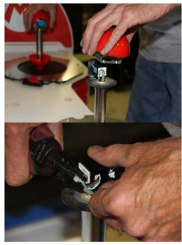
3. Twist light off of button an pull 4 wire plug from underneath.
