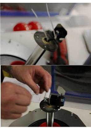
6. Use wire tie to secure wires to back of light button module with existing tie-down.
