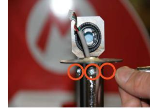
5. Add Heat Shrink to wire between existing gray insulation and plug. Secure with 2 wireties. Reattach button light by twisting back into place.
