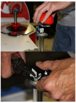
8. Twist light off of button an pull 4 wire plug from underneath.
