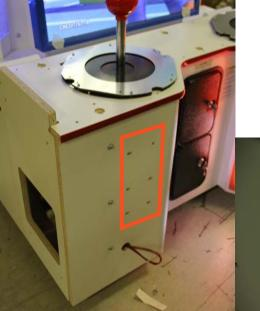
7. With a short philips screwdriver, remove the 4 screws located under the ball of the the joystick. It should drop down. Do this and the next 2 steps for both joysticks.
