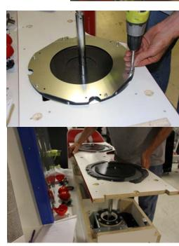
11. Next to the joystick box, remove the two screws. Now you should be able to lift straight up on the joystick to raise entire joystick housing. Take care to free up wires from hooks while you lift to avoid pulling wires out of the plugs.
