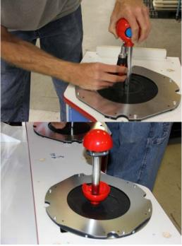
2. Lift off top of joystick ball and set aside. With wire cutter, remove zip tie. Be careful not to cut any wires.
