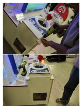
4. Remove 5 screws on each plastic joystick cover and remove. Remove center plate as well.
