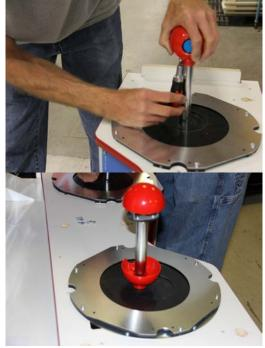
7. Lift off top of joystick ball and set aside. With wire cutter, remove zip tie. Be careful not to cut any wires.
