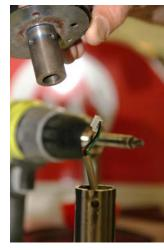
9. For right and Left, remove 4 screws around shaft of joystick and lift of top.
