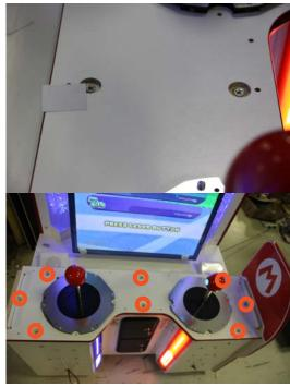
6. Remove 6 screws on the front under the joystick and 2 screw in between lighted panel and coindoor.
