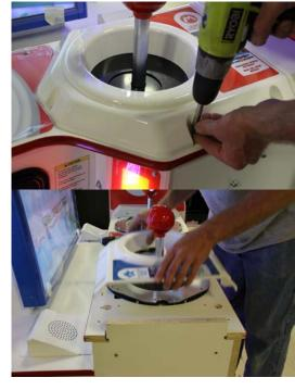
5. Remove white decal from under center plate to reveal 2 screws. Proceed to remove 8 top screws(circled in red) to free up top counter.
