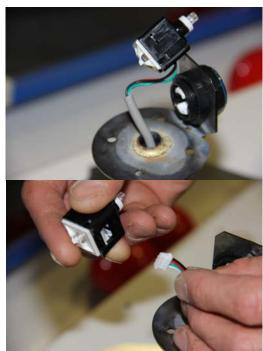
4. Remove 4 screws around joystick shaft and discard. Replace with shorter 4x10mm screws with LockTite or similar threadlocker.
