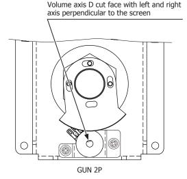
FIG. 11-2b X Axis (Left and Right) Volume
