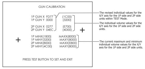
FIG. 9-3c02 Calibration Screen
