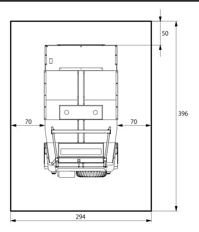
FIG. 2 Installation and operation area (cm)
