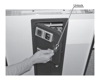
Grab both sides of the switch with your fingers and rotate it approximately 45 degrees in the direction of the arrow in the figure to take it off.
