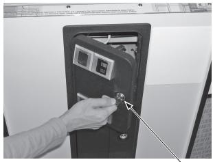
Grab both sides of the switch with your fingers and rotate it approximately 45 degrees in the direction of the arrow in the figure to take it off.
