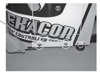
The controller cabinet has 4 casters and 4 adjusters. Make sure that all the adjusters are in contact with the floor directly. Use a wrench to set adjuster heights so that the controller cabinet will stay level.
