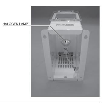
Attach the ground terminal, flat washer, spring washer, and hexagon nut to the threaded shaft inside the halogen lamp cover in that order, and fasten it in place.
