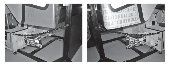
Affix the chain holder B to the controller cabinet and fasten it in place with the screw and the bush.
