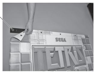
7 Insert the shanks on the front center banner sash into the counter-sunk holes on the roof panel. Another person should fasten it in place with the 5 truss screws removed in Step 4 of "6-1-2 Attaching the Roof Panel."
