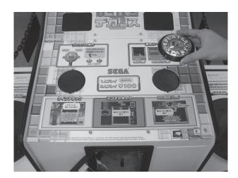
Remove the 8 tamperproof screws and take off the lower instruction plate (transparent plate).
