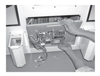
Disconnect the 4 connectors connected to the SystemSP board.
