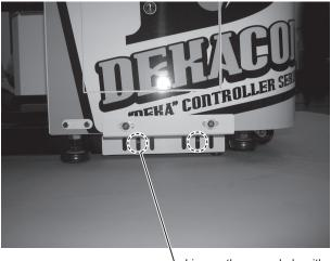
Line up the screw hole with the second elongated hole from the outside.
