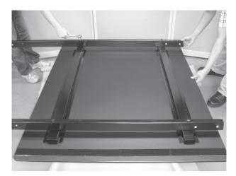
Attach the roof bracket L (DKC-0673) to the post frame. Insert the protruding part of the screw holes on the post frame into the holes on the bracket, and lightly fasten it in place with 2 hexagon bolts.
