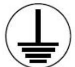
Indicates a "Protective Earth Terminal". Before operating the equipment, be sure to correctly connect it to an Earth point.
